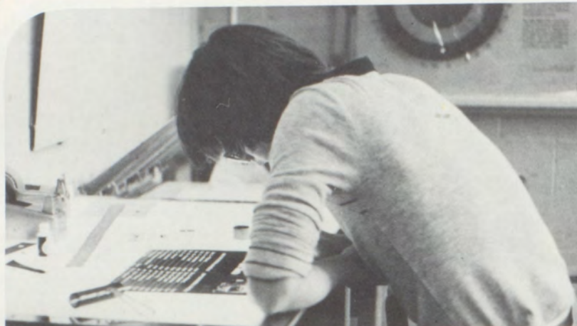
Bert Quisenberry is opaquing a negative in Charles Belts' printing class. This will keep small spots from showing on printed materials.
