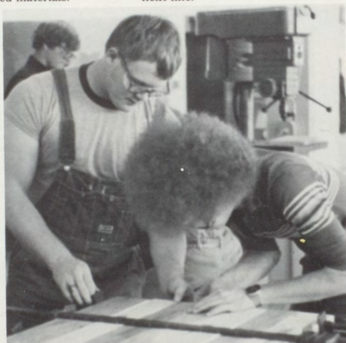
Chip Schuler tries to even up the ends of the boards before he cuts them.
