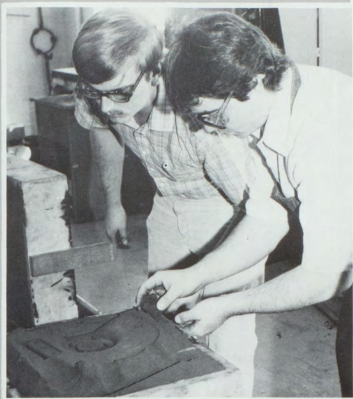
ABOVE: Tim Knoles and Tim Eytcheson, senior, perfect a mold before pouring the metal to make an aluminum guard for a grinder. RIGHT: Jim Hogan figures grades before down cards go out for the fourth quarter. BELOW: Jerry Bellem, Chris Groth, Jimmy Carrol, Tom Linn, Chris Ashford, Randy Bell, Clinton Greer, Alan Cessna, Mike Hugo, Tom Korhn. VO TECH STUDENTS
