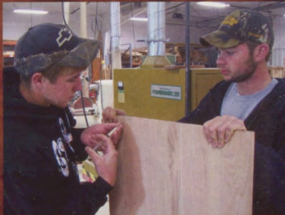
Garrett Gilstrap and Gordon Gartner inject glue into a piece of wood.
